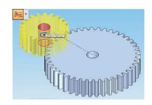
A dedicated motion editor or timeline automatically captures motor events as they are created and allows you to easily control motor properties such as direction, speed and travel. This timeline also provides a graphical interface that allows you to quickly drag and drop motor properties to adjust when a motor should start, or to increase or reduce how long a motor should run.
