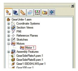
Multiple motors can be applied to the same part. Multiple motors are primarily used so that different motors can be turned on/off in the timeline, for example, a motor could be turned on from zero to 10 seconds to move a component in the x-direction, then turned off and another motor turned on to move the component in the y-direction.
