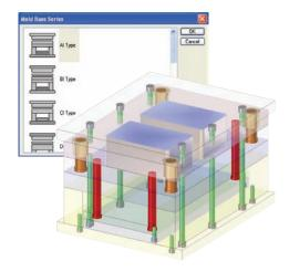
You can easily create a pattern of the blocks for multi-cavity molds. Solid Edge Mold Tooling lets you quickly reorient the individual blocks and automatically center them in the mold base for a balanced runner system.
