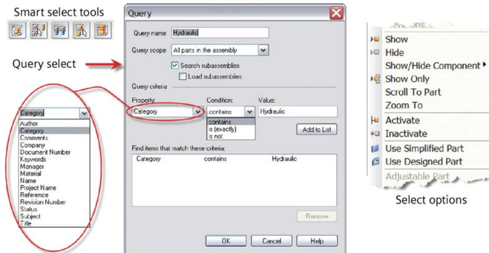
Figure 9: Solid Edge selection tools, options and display configurations provide quick, convenient ways to select and choose component displays.
