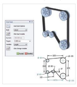
constraints and the system solves for the desired parameter – hence the term Goal Seek. Solid Edge computes and stores the most common measurements such as distance, angles, perimeters and areas for fast problem definition, and includes intrinsic functions for doing math and trig operations needed in complex equations.
