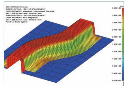
Displacement results from a metal forming example. A planar sheet is formed into an S channel.
