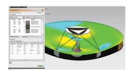
NX Laminate Composites also computes core ply transverse shear failure indices, strength ratios and margins of safety using allowable shear stresses in the 23 and 13 directions.
