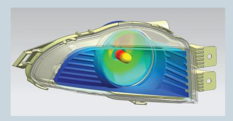
NX Advanced Thermal continues Siemens' long heritage in thermal simulation and leverages the same technology that underpinned the I-deas TMG solution. NX Advanced Thermal adds a rich feature set to the powerful simulation technology of NX Thermal. Intended for tackling complex thermal physics and challenging thermal management problems, NX Advanced Thermal offers the same best-in-class level of integration within the NX preprocessing, postprocessing and simulation tools.
