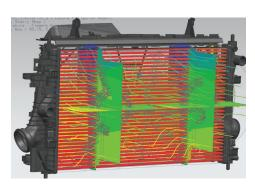
You can conduct coupled thermo-flow analysis without the need to transfer data between multiple software tools.
